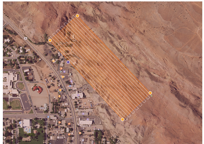
Figure 6. Example of land survey flight plan
