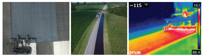
Figure 8. UAS surface treatment inspection (visible and IR)
