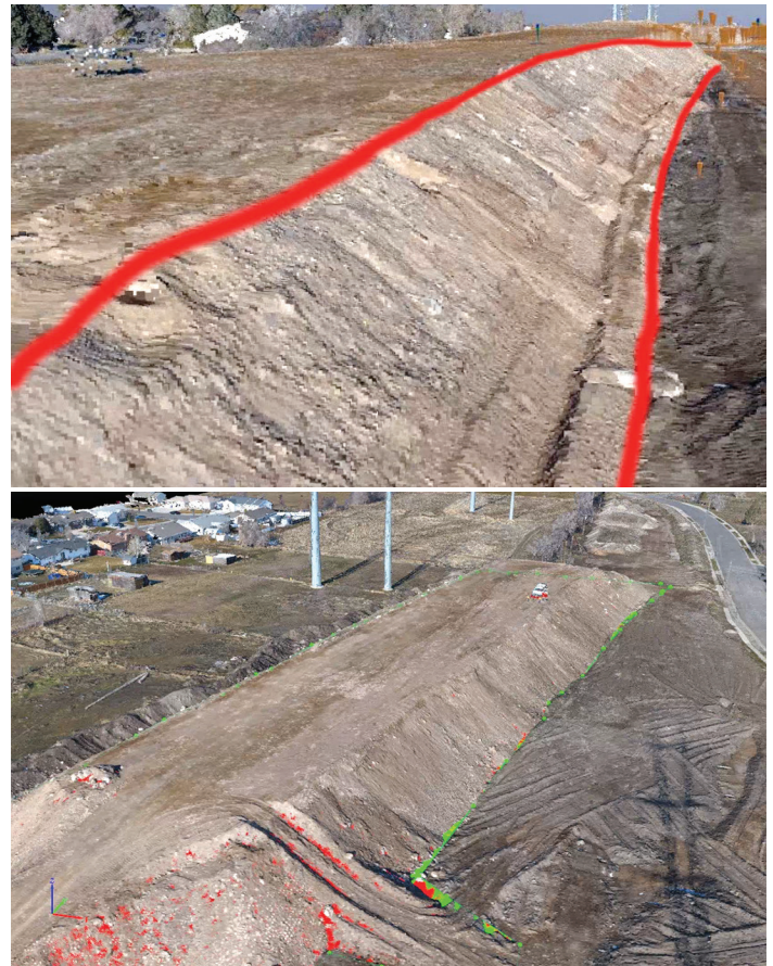
Figure 10. Breakline survey (top) versus point cloud (bottom)
