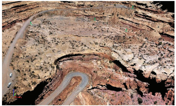
Figure 1. Moki Dugway, Utah landslide 3D point cloud collected using UAS photogrammetry
